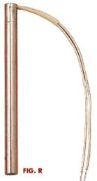
Figure R is used when spacing requirements are limited. See chart below for the additional dimension the Mighty Watt Plus adds to the sheath length of stock items. When ordering non-stock Fig. R, specify the overall sheath length. High temperature (850° F/450° C) leads are fully flexible from the exit of the sheath. 12" lead wire is standard. Specify additional length.
